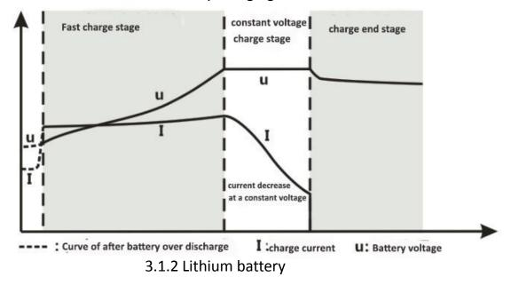
• Trickle pre-charge stage: at the beginning of charging. If the battery voltage is too low, in order to protect the battery, to avoid large current impact caused damage to the internal structure of the battery. The controller will charge battery in a small current. And will enter fast
